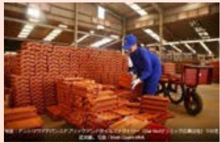
Brick & Roof Tile Factory Manufacturing processes generate about 5 to 7% defective products, which then become waste.
