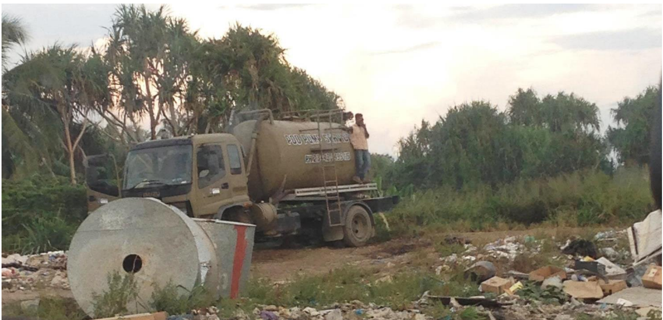
Figure 34: Septic tank collection truck pumping effluent into the Honiara Landfill (Photo: Trundle)
