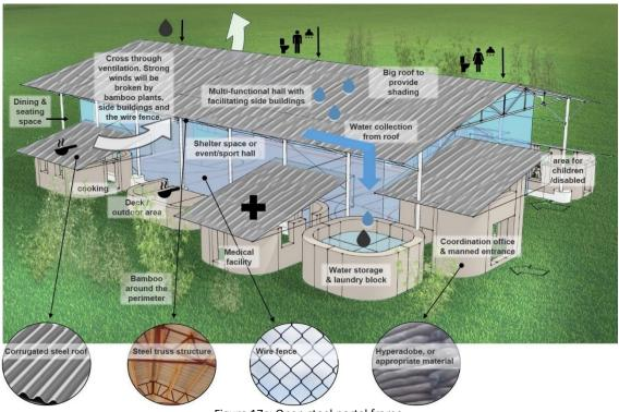
Figure 17c: Open steel portal frame Figure 17: Conceptual designs for the proposed evacuation centre
