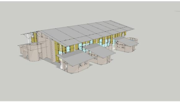
Figure 17b: Steel portal frame construction with bamboo curtain
