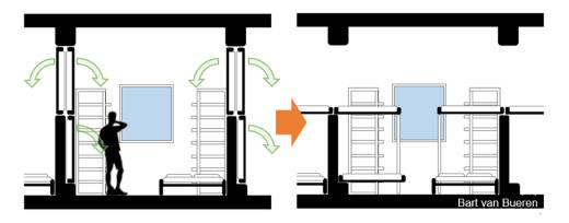
Figure 13: Concept of bunkbeds in the wall of a hotel room, Source: van Bueren (2019).
