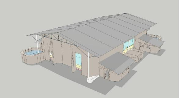
Figure 17a: Steel portal frame construction with concrete block walls
