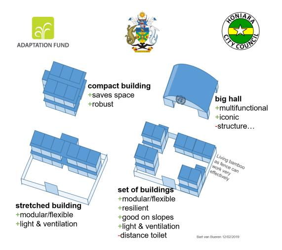
Figure 11: Four different building typologies for evacuation facilities, source: van Bueren (2019)
