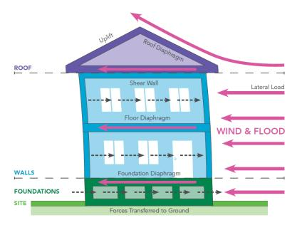
Figure 22: Wind and flood load distribution (Source: Federal Alliance for Safe Homes, 2016)
