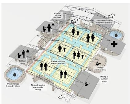
Figure 19a: Internal layout option with moveable partition walls
