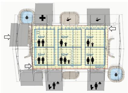
Figure 19b: Internal layout option with moveable partition walls Figure 19: An example of layout plan of the proposed evacuation centre
