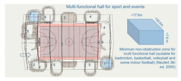
Figure 18: Floor plan configurations of pilot concept design of a big multifunctional hall
